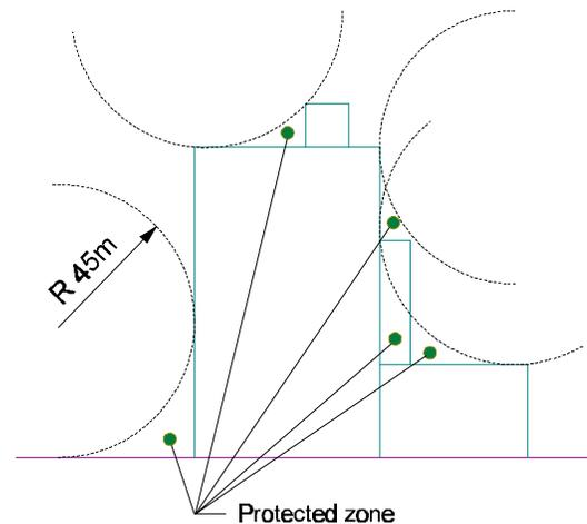
Figure 2. Protection design using Rolling Sphere Method
